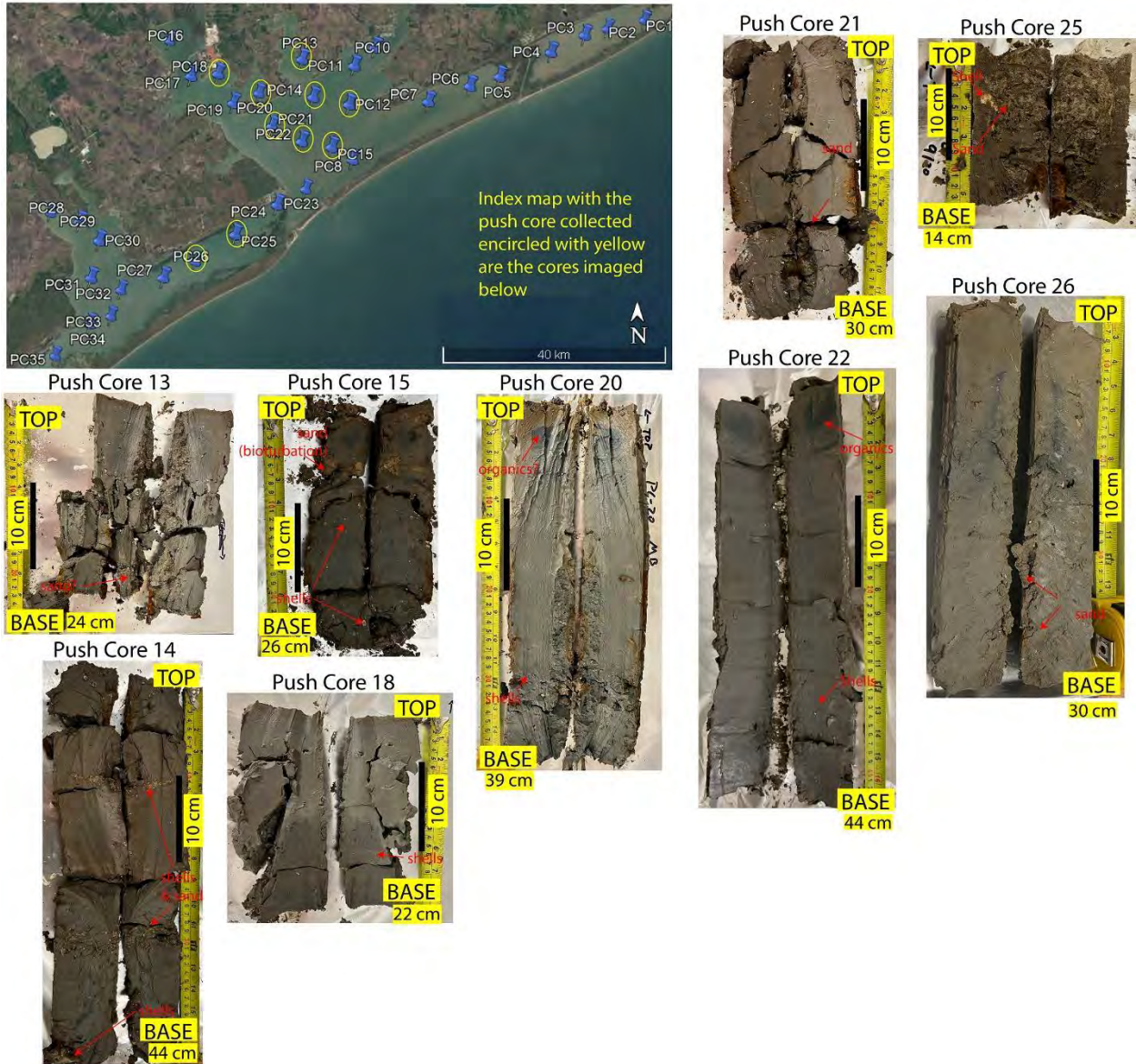
Figure 30. Photos of the sediment cores 13, 14, 15, 18, 20, 21, 22, 25, 26 from Matagorda Bay. Top left map indicates the location of the cores. Cores are dominated by muddy sediments with two exceptions, cores 24 and 25, which are muddy sands. These cores are located proximal to Pass Cavallo, where a flood tide delta composed of marine sands dominates the area. Well preserved and obvious bioturbation filled with sand is visible in core 15.
