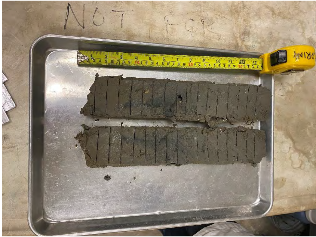
Figure 22. Sediment core (San Antonio Bay site 26) subsampling (2cm interval).
