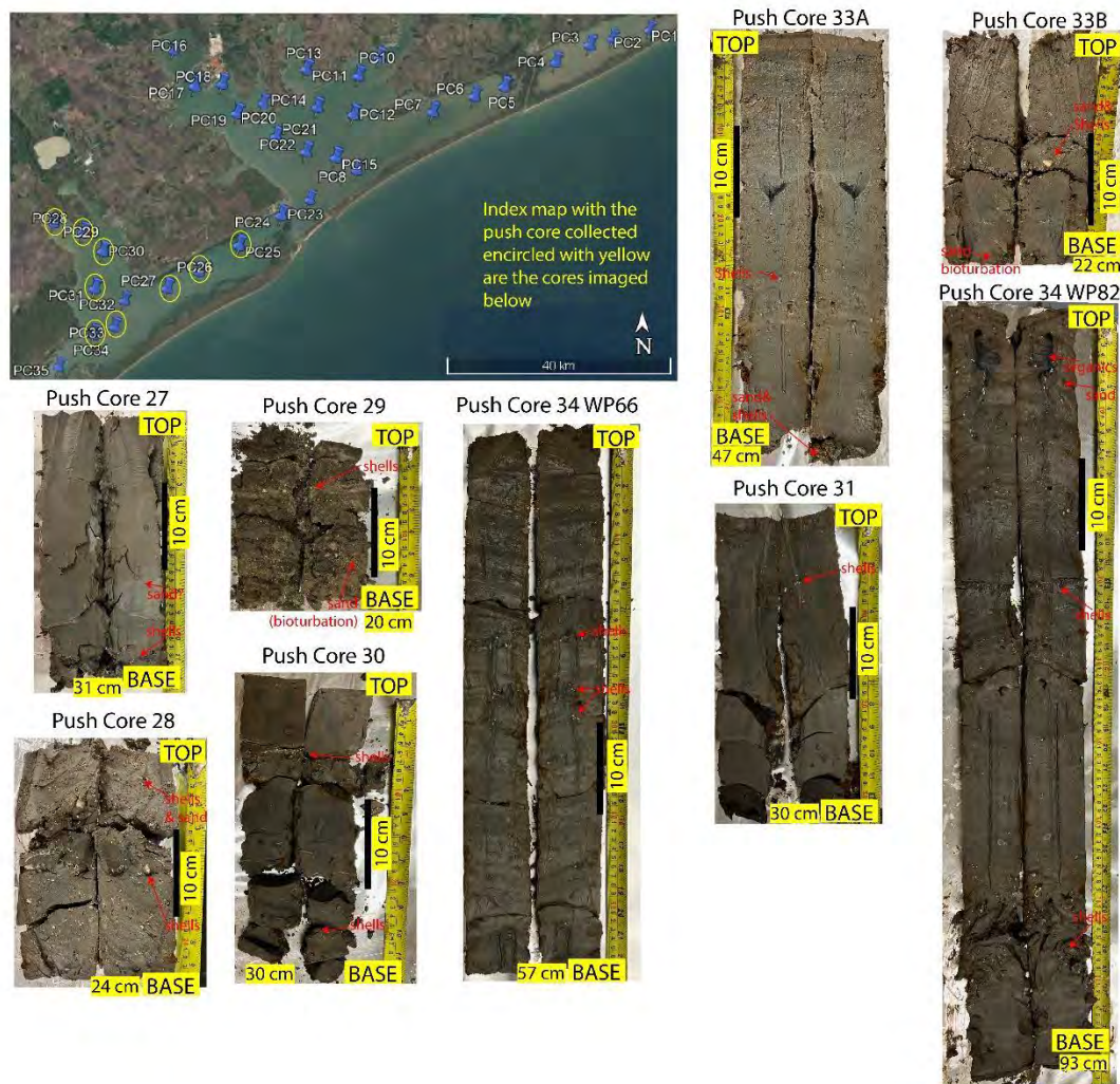
Figure 31. Photos of the sediment cores 27, 28, 29, 30, 34 WP66, and 34 WP82 from San Antonio Bay. Top left map indicates the location of the cores. Note that core 29 has multiple sand intercalations. Cores 30 and 34 WP82 have some clear shell fragments and (probably?) sand-rich intervals indicating higher energy flow events.
