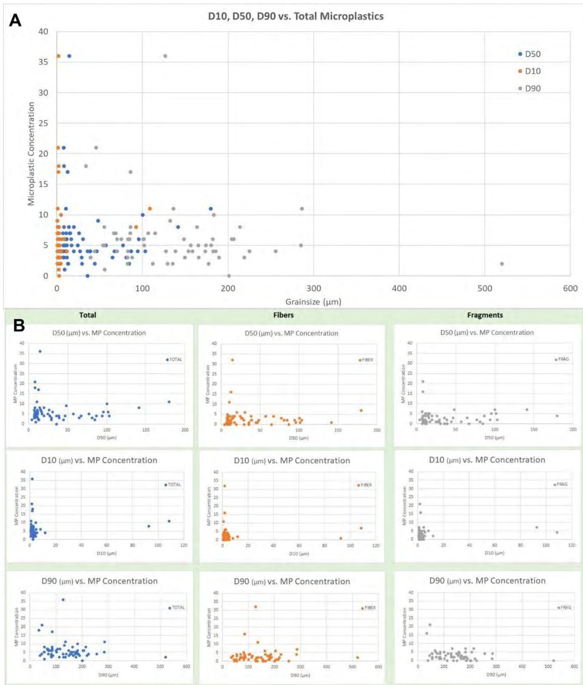
Figure 44. Sediment grain size versus microplastic (MP) concentration. A – All microplastics found plotted against D10-D50-D90 values. B – Microplastics concentration separated by type (fiber, fragments) versus grainsize values at D10, D50 and D90.
