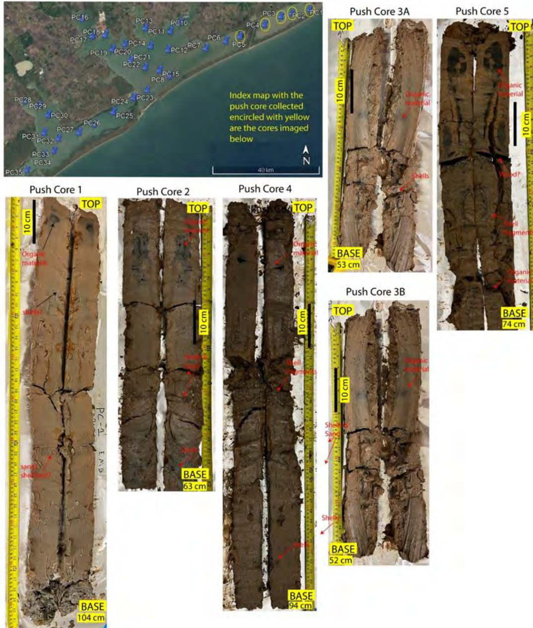
Figure 28: Photos of sediment cores 1, 2, 3A, 3B, 4, and 5 from East Matagorda. The top-left map indicates the location of the cores. Cores are dominated by muddy sediments with some thin laminae of sand or shells. Note that cores 4 and 5 have more organic content (fragments or dark grey mud) and are also located closer to the Colorado river outlet, which is the source for the organic material.
