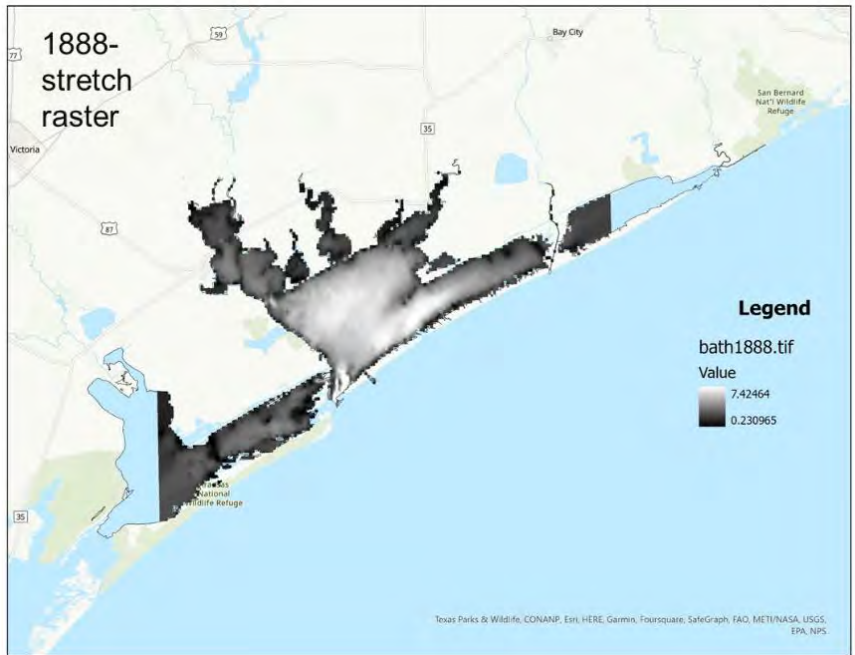
Figure 56. Digitized and re-gridded navigational bathymetric chart from 1888, depth units in meters.
