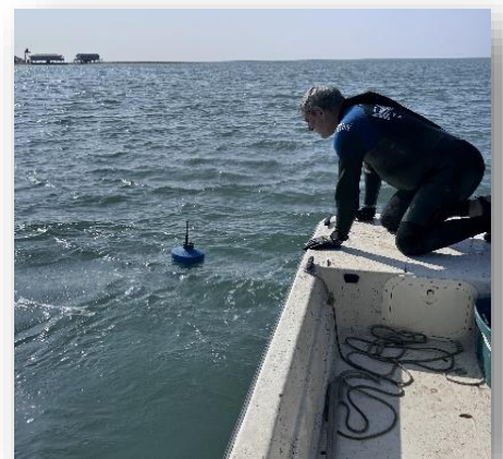
Dr. Philippe Tissot, TAMU-CC installing temperature monitor in Espiritu Santo Bay.
