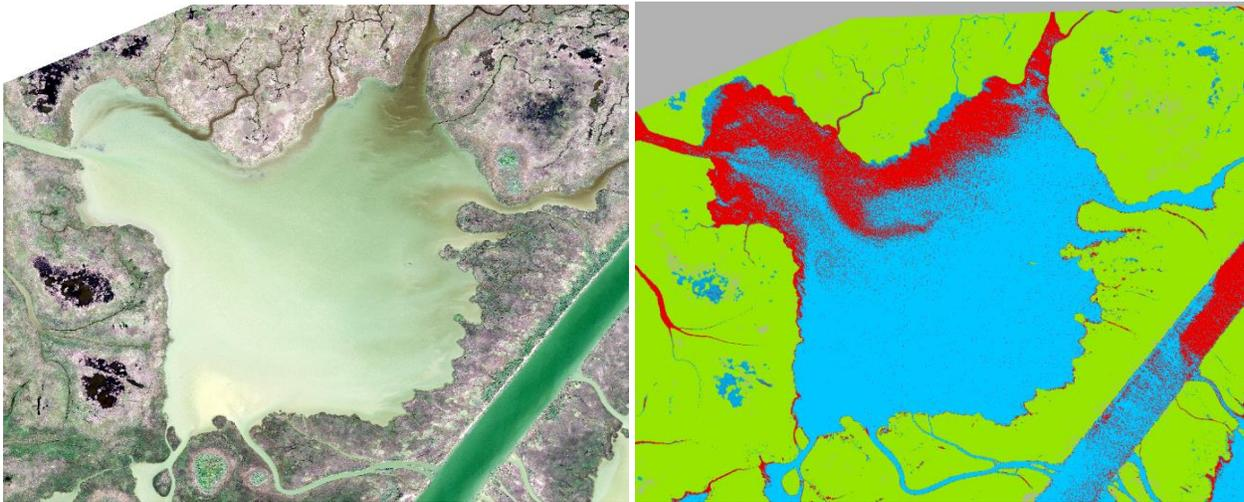
**Figure 1.** High resolution satellite imagery from November 2022 and groundcover classification to extract oyster bed areas for comparison against sonar imaging.
