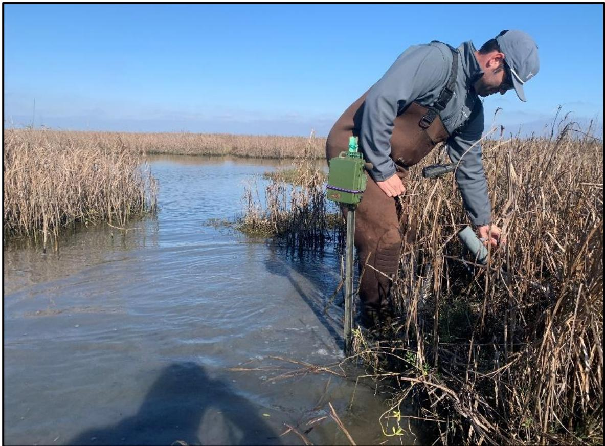
**Figure 19.** Typical view of a deployed Song Meter SM4 Bioacoustic Recorder.
