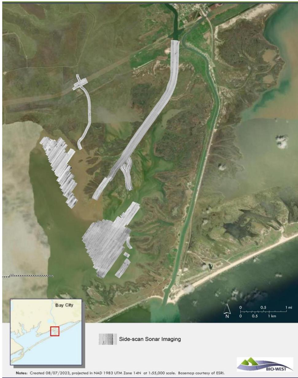
**Figure 2.** Side-scan Sonar imaging within the study site area of the Colorado River Delta.
