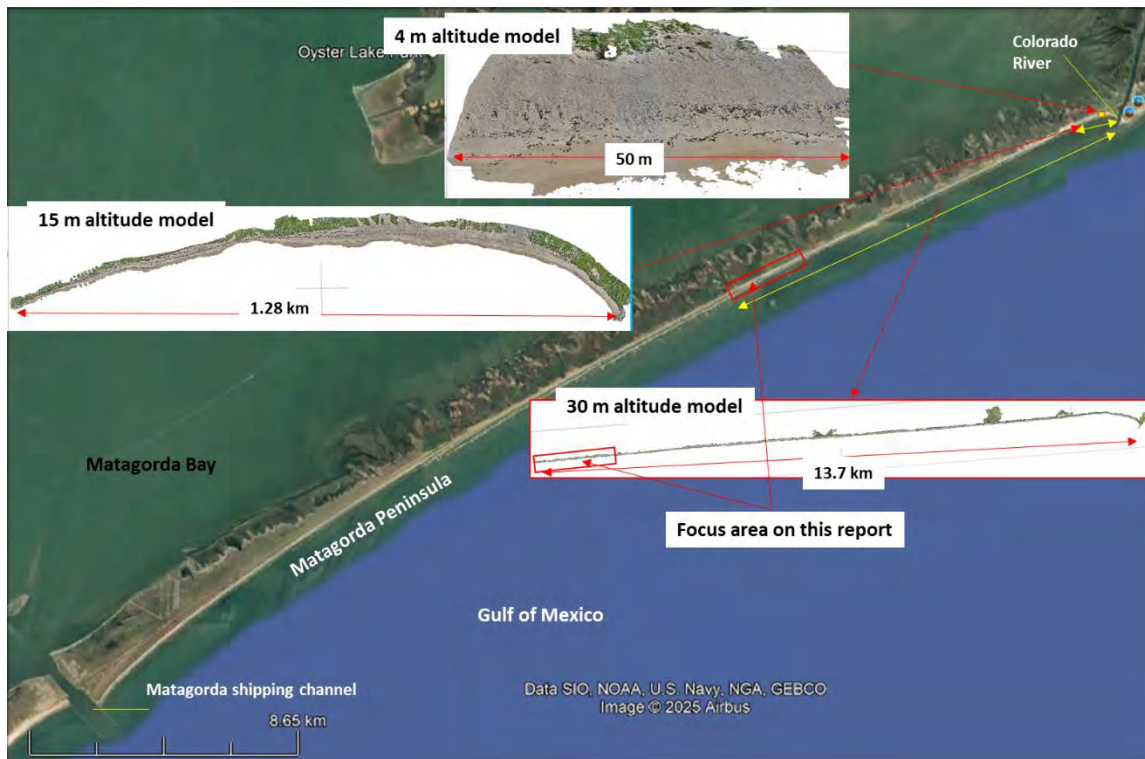
Figure 1. Map of the Matagorda Peninsula showing the area of UAV imagery collected at different altitudes for comparison.
