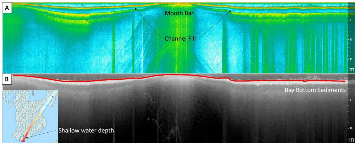
**Figure 2.** Example of CHIRP (A) and Downscan sonar (B) data collected along the Colorado Delta distributary channel.
