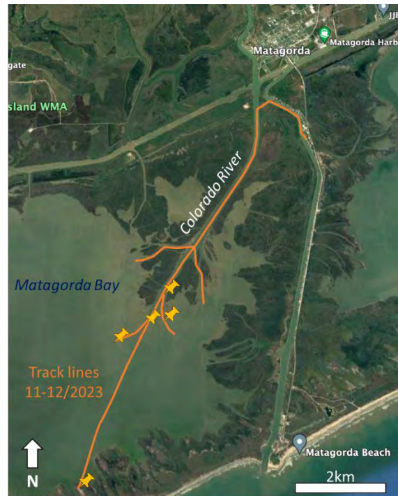
Figure 18. Data collected during December 2023 field work. Lower left photo show sediment data collected in delta front area of Colorado. On the right the lines of Chirp data and sediment sample locations.
