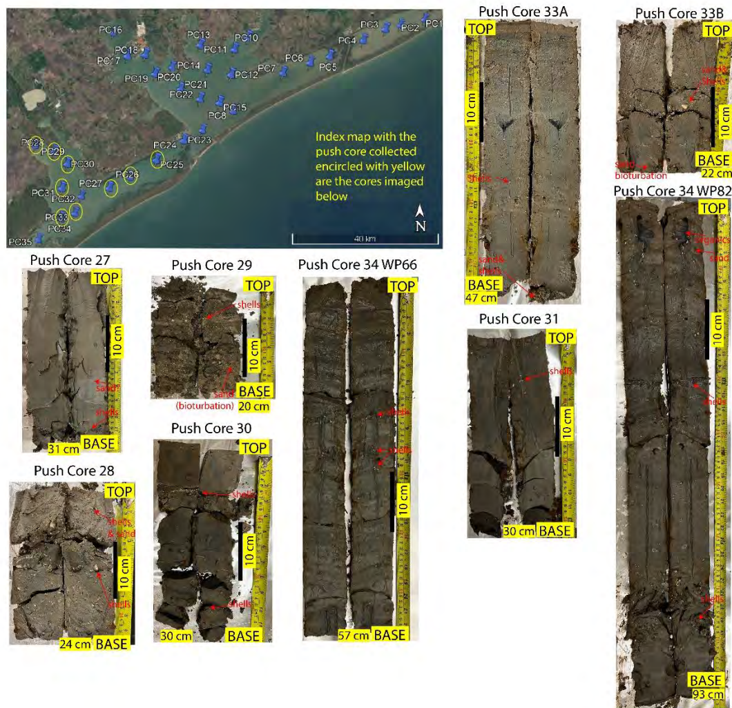
Figure 4. Photos of the sediment cores 27, 28, 29, 30, 34 WP66 and 34 WP82 from San Antonio Bay. Top left map indicates the location of the cores. Note that core 29 has multiple sand intercalations. Cores 30 and 34 WP82 have some clear shell fragments and (probably?) sand rich intervals indicating higher energy flow events.
