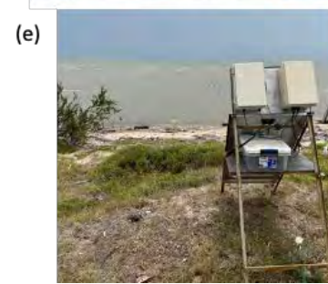
(a) Sensor set up on the tripod, (b) the tripod during deployment, (c) the tripod after deployment, (d) the ADCP velocity sensor post-deployment, (e) the computer station used to communicate with the X-bee wave sensors, and (f) the linked sonar and survey-grade GNSS system, attached to the side of the boat.
