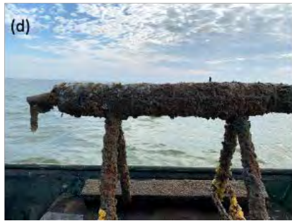
(a) Sensor set up on the tripod, (b) the tripod during deployment, (c) the tripod after deployment, (d) the ADCP velocity sensor post-deployment, (e) the computer station used to communicate with the X-bee wave sensors, and (f) the linked sonar and survey-grade GNSS system, attached to the side of the boat.
