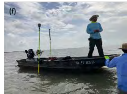
(a) Sensor set up on the tripod, (b) the tripod during deployment, (c) the tripod after deployment, (d) the ADCP velocity sensor post-deployment, (e) the computer station used to communicate with the X-bee wave sensors, and (f) the linked sonar and survey-grade GNSS system, attached to the side of the boat.
