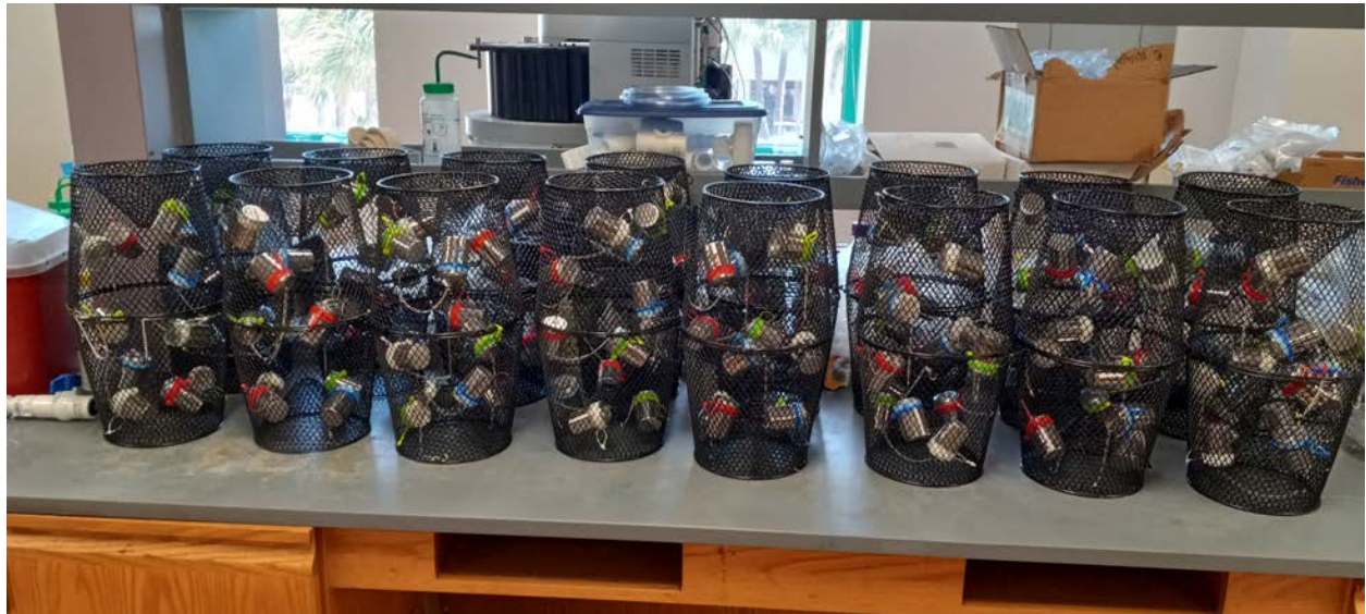
Figure 1: Hg Adsorption study - samplers comprising four different polymer types in triplicates for each sampling site for four weeks.
