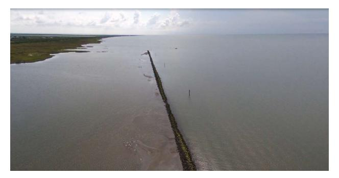
Figure 17. Sediment accumulated behind the Schicke Point living shoreline constructed in May 2017 (July 6, 2018, 14 months post-construction). Marsh in the background beyond the living shoreline is the marsh proposed for protection and restoration in this proposal.
