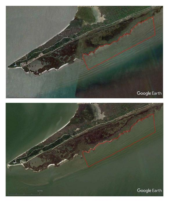
Figure 15. Photograph above is dated December 2, 2016, 18 months before completion of the living shoreline. Photograph below is dated December 1, 2018, about 6 months after completion of the living shoreline. Extensive areas of sediment accumulation can be seen behind the living shoreline along with increased plant coverage of shell hash berms. The area outlined in red is the Matagorda Bay shoreline to be protected by the proposed project.
