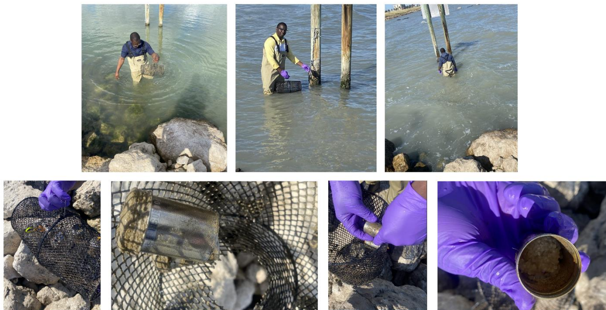
Figure 2: Pilot Sampling to determine environmental rates of Hg sorption to new plastics conducted between October 5-26, 2022.
