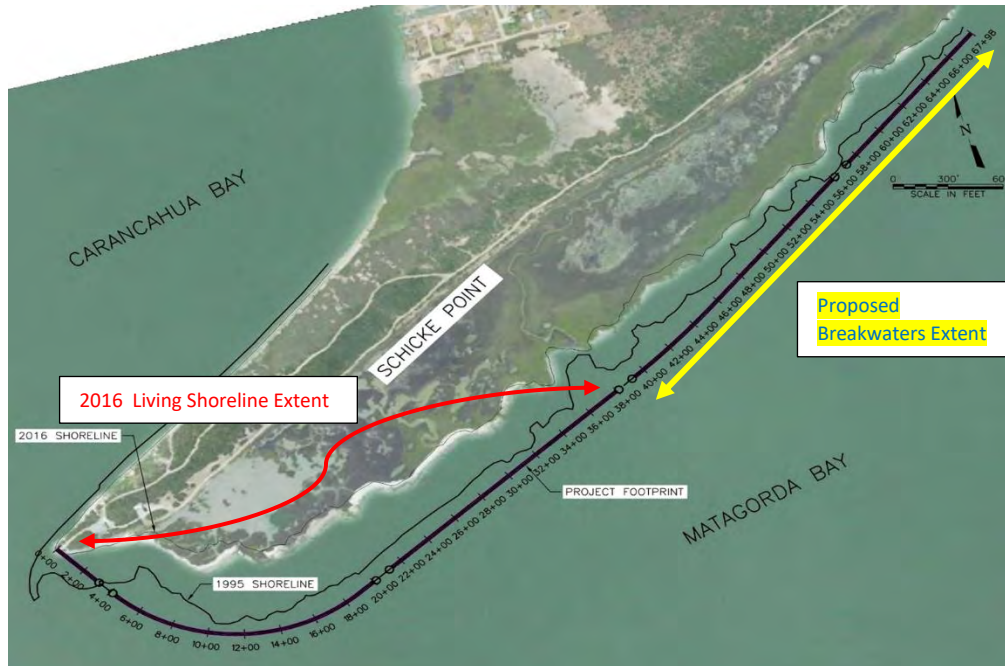
Figure 1. The figure shows the permitted living shoreline structure (USACE SWG-2016-00111). The living shoreline structure and proposed breakwater extension roughly follows the 1995 shoreline.
