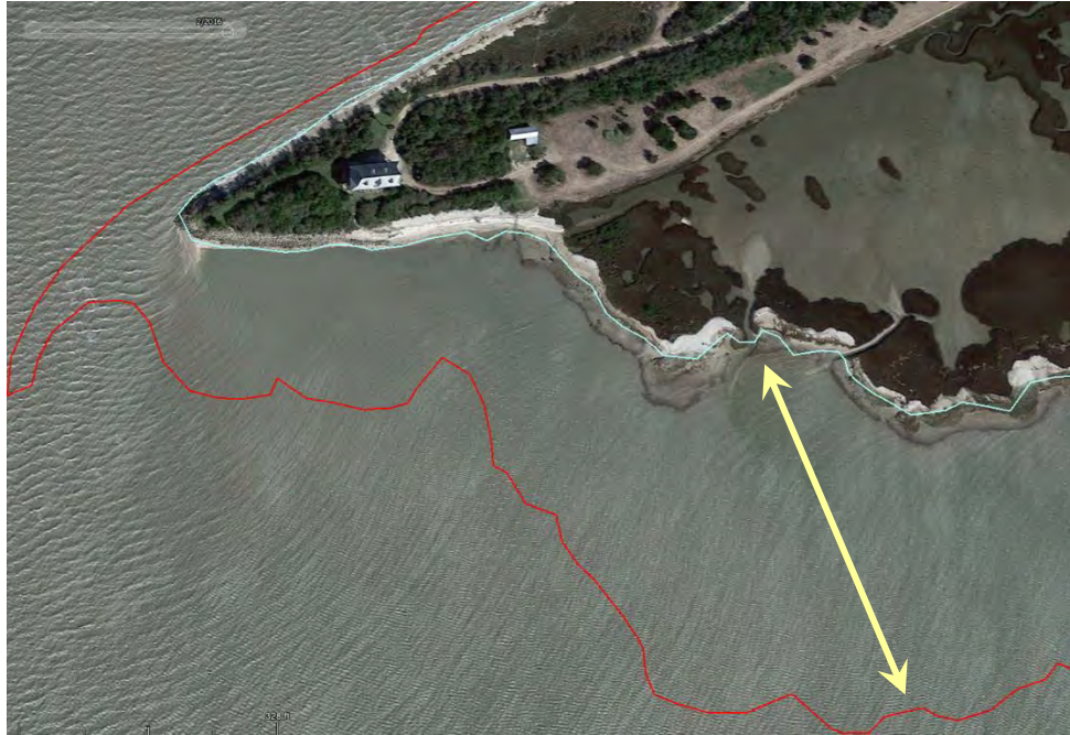
Figure 3. The figure shows the 1995 shoreline (red) and aerial imagery from 2016. Schicke Point had experienced approximately 400 feet of shoreline loss within the span of 11 years.
