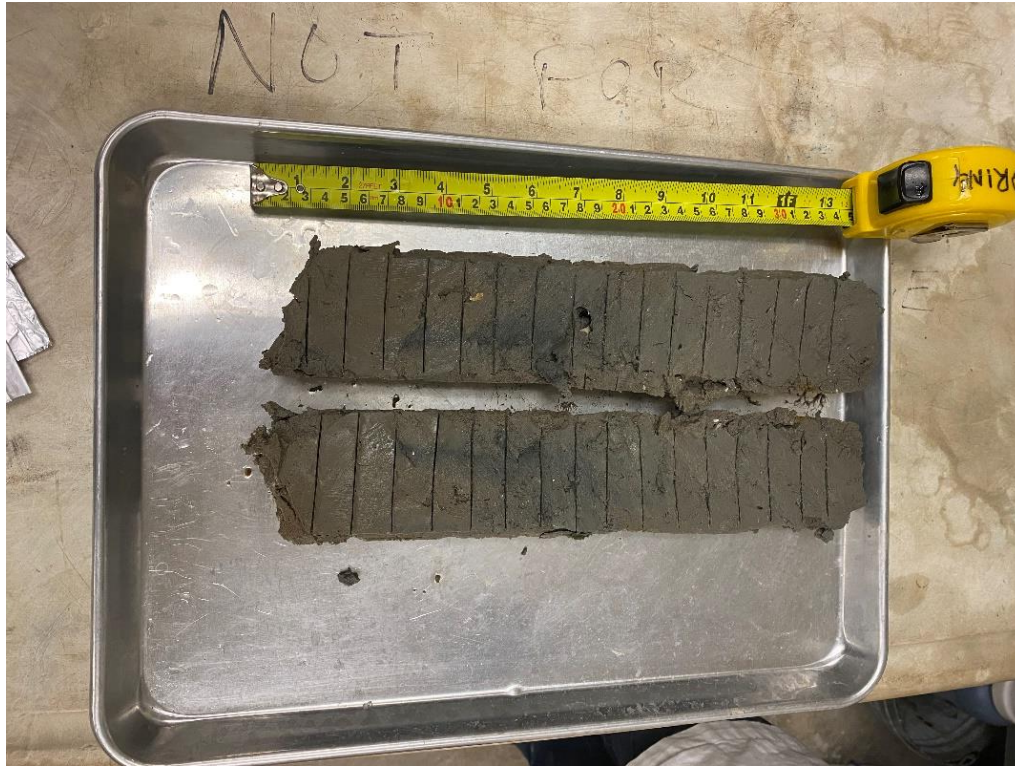
Figure 4. Sediment core (San Antonio Bay site 26) subsampling (2cm interval).
